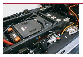
Specially designed Bucher Battery Pack with superior lifetime and minimal memory effect. Made with high quality automotive prismatic Li-ion NMC cells, managed through an automotive battery management system, the battery is placed in a shock, water and dust-proof case. The Bucher Battery Pack is maintenance-free and has a sophisticated repair concept for maximum safety. Due to the electric drive concept of the sweeper, maintenance and service costs in general are kept low.
