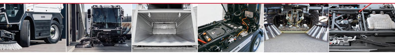
4 wheel steering 3rd brush 5.6 m³ Hopper 137 kWh Bucher Battery Pack Wide suction intake 118 kW, Euro 6 emission diesel engine
