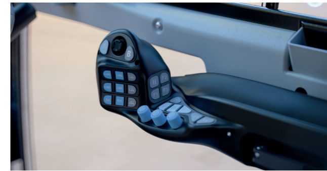
Smart-Con armrest Multi-functional armrest with smart start function makes it possible to operate all working functions with one hand.
