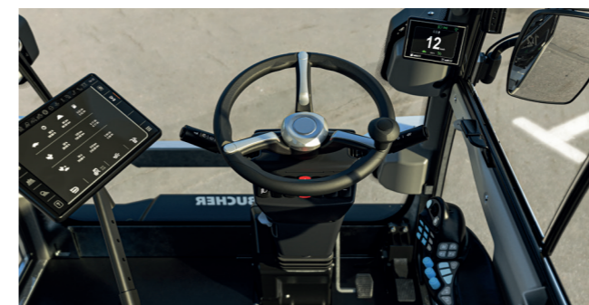
Cab Comfortably suspended, sound-insulated and ROPS tested aluminium cab. Windscreen made of heat-reflecting, curved, low-reflection safety glass.
