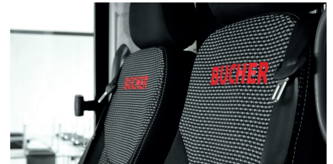
Seats The cabin can be equipped with two fully fledged driver seats with headrests and 3-point safety belts to offer not just a comfortable driving experience, but also an ergonomic workstation (optional).
