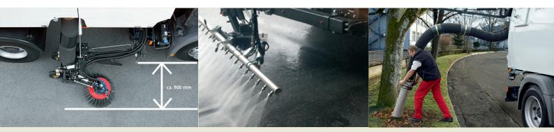
**Telescopic pick-up unit** The telescopic pick-up unit can be extended by an additional 250 millimetres to obtain the best cleaning results.
